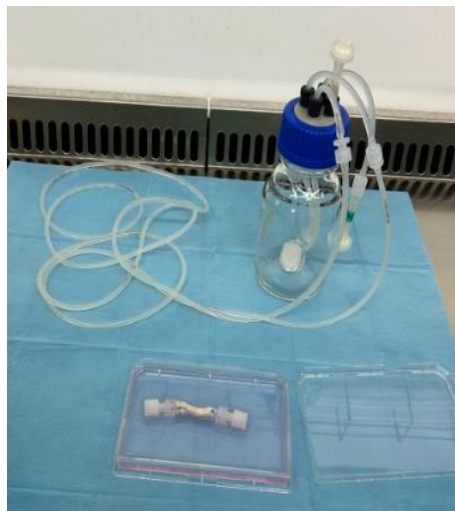
Figure 2 - In vitro repopulation: The cells are seeded in the lumen of the bile duct and then a in-house developed bioreactor is used to mimic the in vivo flow to stimulate cell spreading and proliferation.
